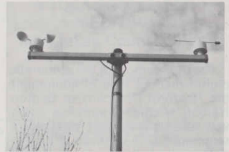
Figure 5. The anemometer/wind vane apparatus should be mounted on a mast and should be located away from or above any trees or other obstacles in the area.
