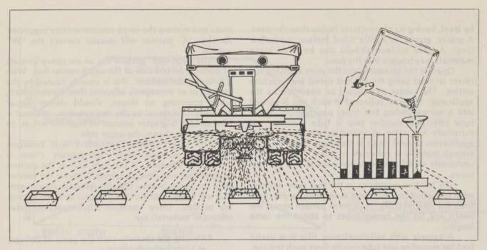
This drawing gives a general idea of how to arrange your collection pans and the cylinders used to measure the levels. Actually, though, you will need 11 or more trays, not the seven shown in the drawing.
