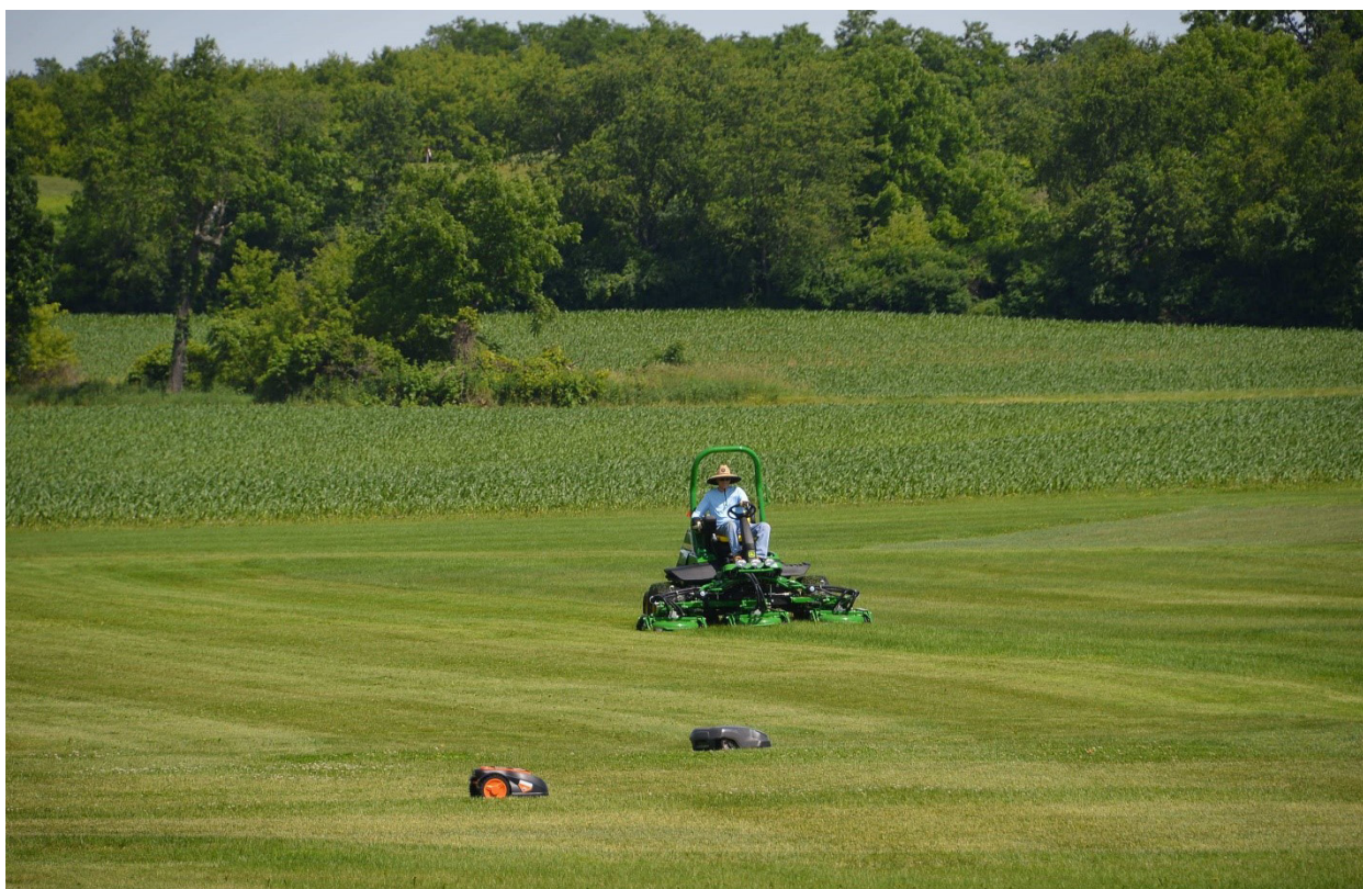
Figure 1. Two of the consumer grade robotic mowers are shown in the foreground with the commercial grade traditional mower operating in the background. (Photo: Micah Woods)
