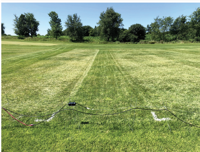
Figure 3. Picture showing differences in mowing quality for Robomow (left), Honda push mower (center), and the WORX robotic mower (right). The cords in the foreground are providing power to the charging stations.
