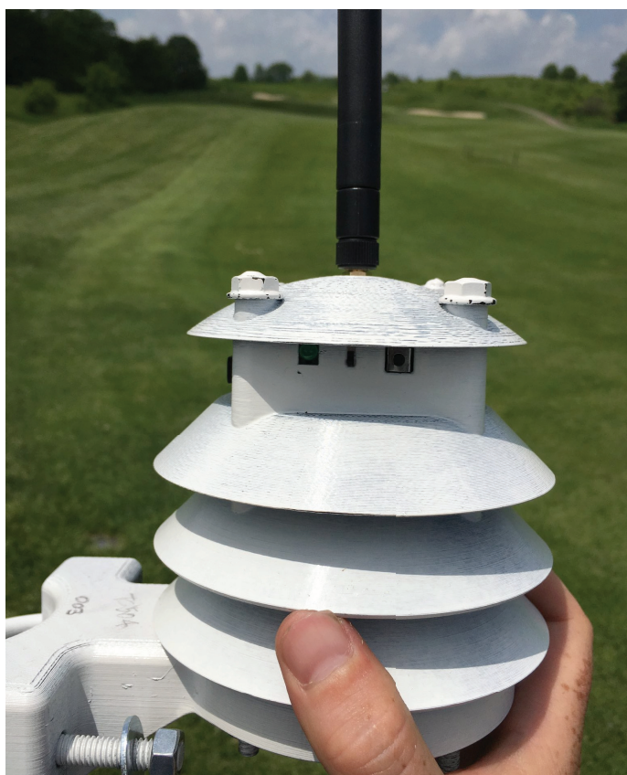
Figure 3: These small weather sensors with the Smith-Kerns Dollar Spot Model embedded in them were tested at the OJ Noer and University Ridge in 2019. We had some technical difficulties but new ones will be ready in time for 2020.
