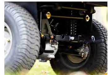
Coil-over shocks suspension for smooth operation
