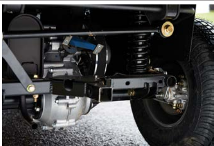
Coil-over shocks suspension for smooth operation
