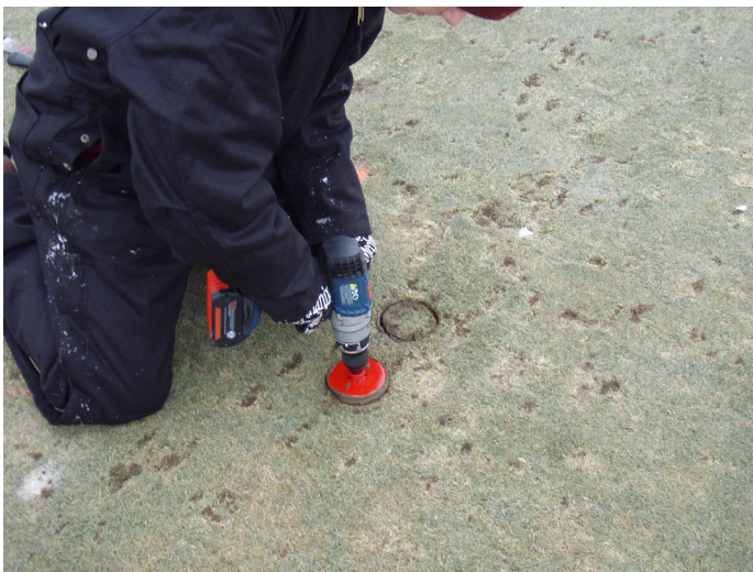
Photo 3: Once the soil had frozen, cores were sampled using a power drill with 4-inch holesaw attachment.
