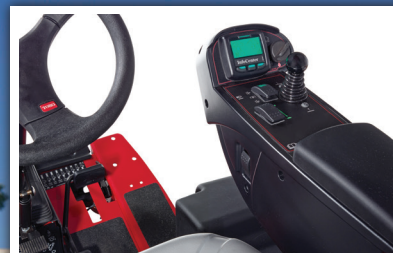
The LCD InfoCenter™ provides system information, diagnostics & service reminders
