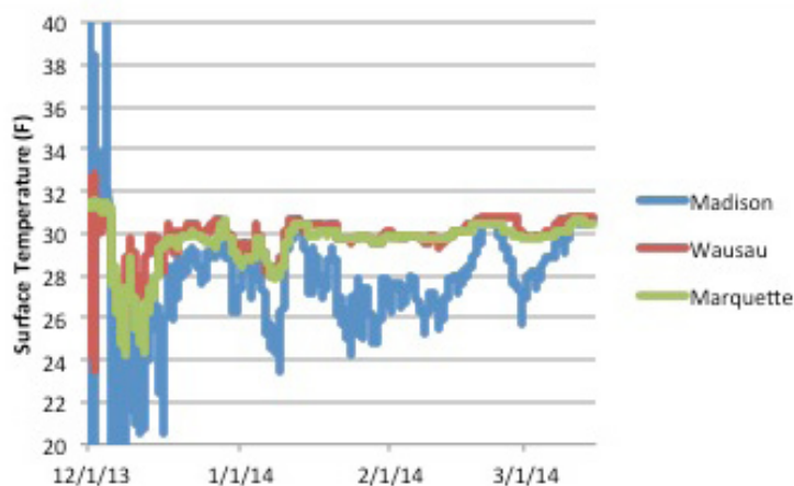
Figure 4: Surface temperatures under snow cover at Tumbledown Trails GC in Madison, WI; Wausau CC in Wausau, WI; and Marquette CC in Marquette, MI throughout the winter of 2013-2014. (Figure originally appeared in the August, 2014 issue of Golfdom.)
