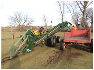
Equipment Mid Valley Golf Course has purchased to allow for a easier drainage project. The trencher is lazer guided to allow for accurate slopes.
