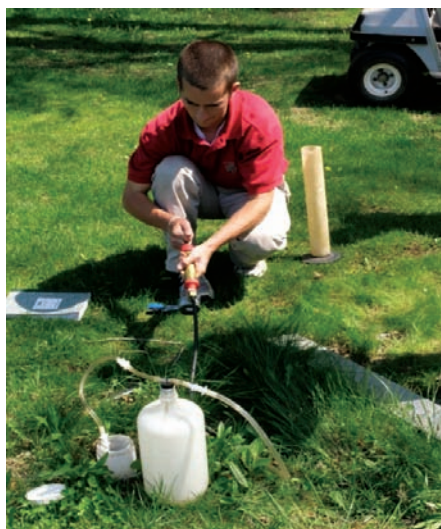
Fig. 2. Graduate student Jake Schneider pumps a lysimeter sample from below-ground of a buffer strip plot at Wisconsin River Golf Course, Stevens Point, WI.
