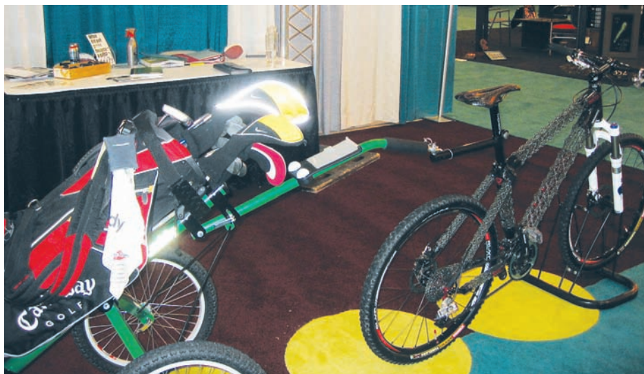
Pedal Power! A hand golf cart designed to be pulled to the course by bicycle.
