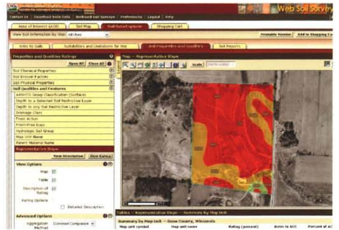
Figure 6. Most of the maps for NR151 can be generated by selecting an AOI, clicking on the "Soil Data Explorer" tab, and then clicking on the "Soil Properties and Qualities" tab
