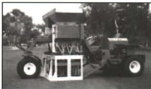
Drill & Fill Aerification
