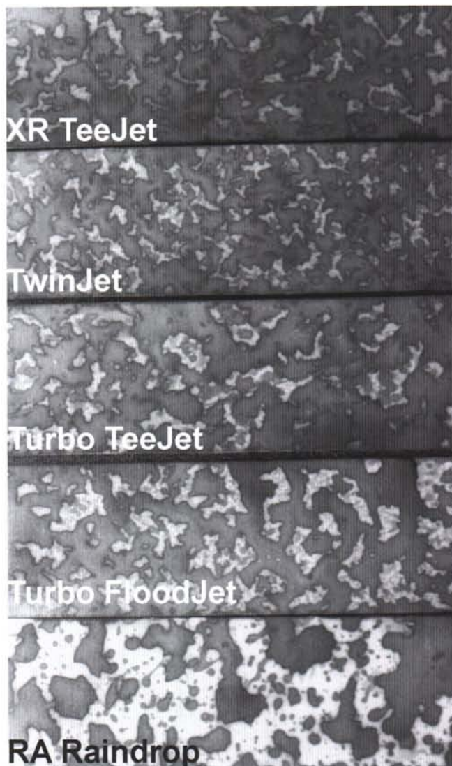
Figure 1. Comparison of nozzle spray pattern using water sensitive paper. The yellow is the original color of the paper and the blue is where the spray pattern landed on the paper.
