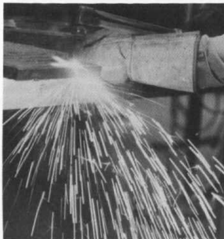
The torch tip is angled up to 90° for making a straight cut on heavy steel plate.
