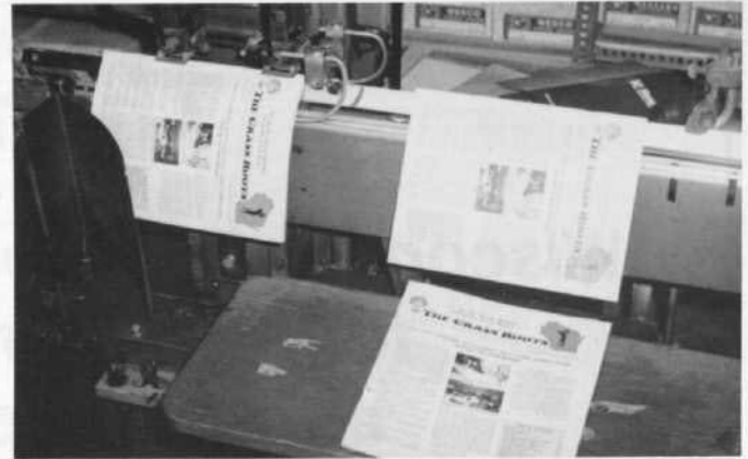
The two-head stitcher staples the booklet together before the final trim is taken.
