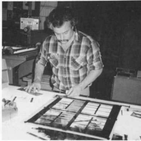
Jim Allhands works at laying the halftones in to the flat for Ransome's 4 page inside spread.
