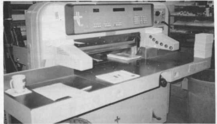
Kramer's computerized Polar cutter takes the final trim off the finished product and "voila" the Grass Roots is completed.
