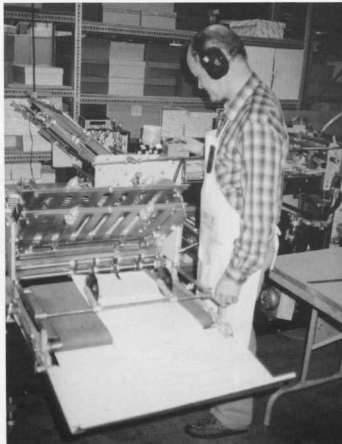
Folder operator, Jon Hayes runs one of the 8-page signatures through the folder in preparation for collating, stitching and trimming.
