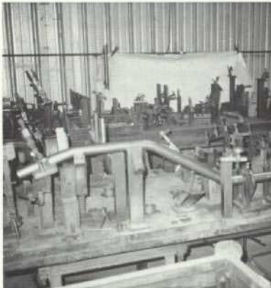
Jigs for frame fabrication.
