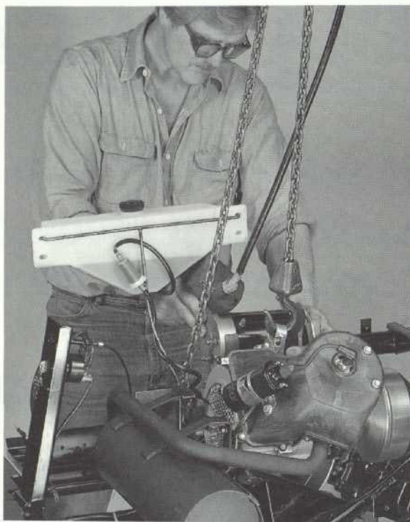
An engine is bolted into the chassis.
