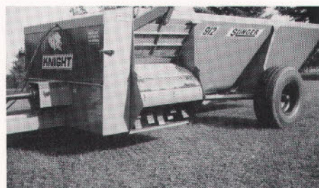
The Knight spreader is an extremely well-built and heavy duty machine. The flail bars you see at the delivery chute each weighs 10 pounds.
