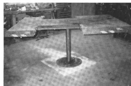
Notice concrete work at base of lift - Van DeHey's unit does require some concrete cutting. This one is in Maple Bluff's shop; Tom Harrison modified the deck to 92"x67" - it is large enough to lift a HF-5.
