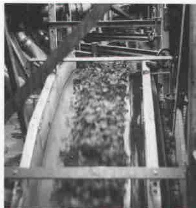
Milorganite going to dryers from filters.
