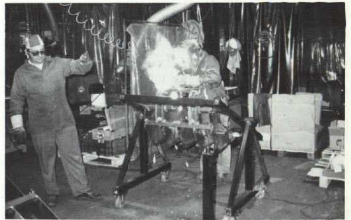
Welding on an assembly for Toro's new Greens Aerator.
