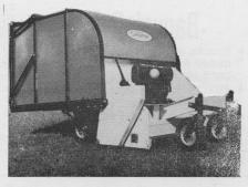
TURF SWEEPER Model 720E Sweeper ROGERS SWEEPERS vary from small self propelled to large 5 cu. yard ca-pacity tractor drawn units.
