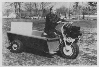
MANEUVERABLE: it turns on itself; 14' clearance circle; 52" turning radius; most maneuverable vehicle on the market. EASY LOADING: ramp tailgate lowers at 10% angle - equipment loaded and unloaded easily by one man. LARGE CAPACITY: it's all carrier - no waste space; #436 Cargo Carrier Capacity -17 cu. ft. approx.; #536 Cargo Carrier capacity - over 23 cu. ft. EASY TO MAINTAIN: no transmission, no differential; no complicated mechanisms.
