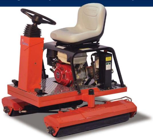
At 605 pounds, it's the lightest riding greens roller made with dual hydraulic roller drive for superior traction and maneuverability.
