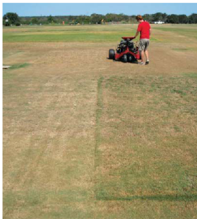
Simulated traffic being applied to deficit irrigation research plots at the Texas A&M Turfgrass Field Laboratory.
