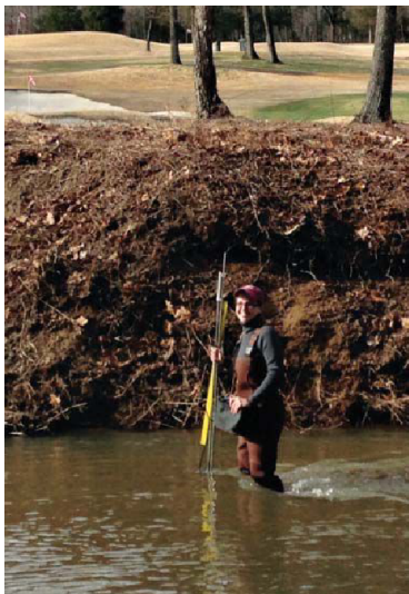
Chantel Wilson measuring velocity at one of the participating golf course research streams, January 2014.
