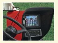
The Capstan® SharpShooter® and the Sharp-Shooter Electronic Control AUTOMATICALLY allow an expanded application rate range from 0.4 to 4.0 gallons per 1,000 sq ft... and operating speeds from 2 to 10 mph... at an operator pre-set pressure necessary to control drift and provide coverage as required. All this is done AUTOMATICALLY with no nozzle tip changes.
