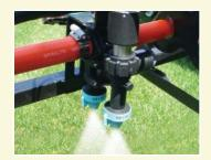
The Star Command System controls the on and off spraying function right at the tip. Shutoff and back on is instantaneous.
