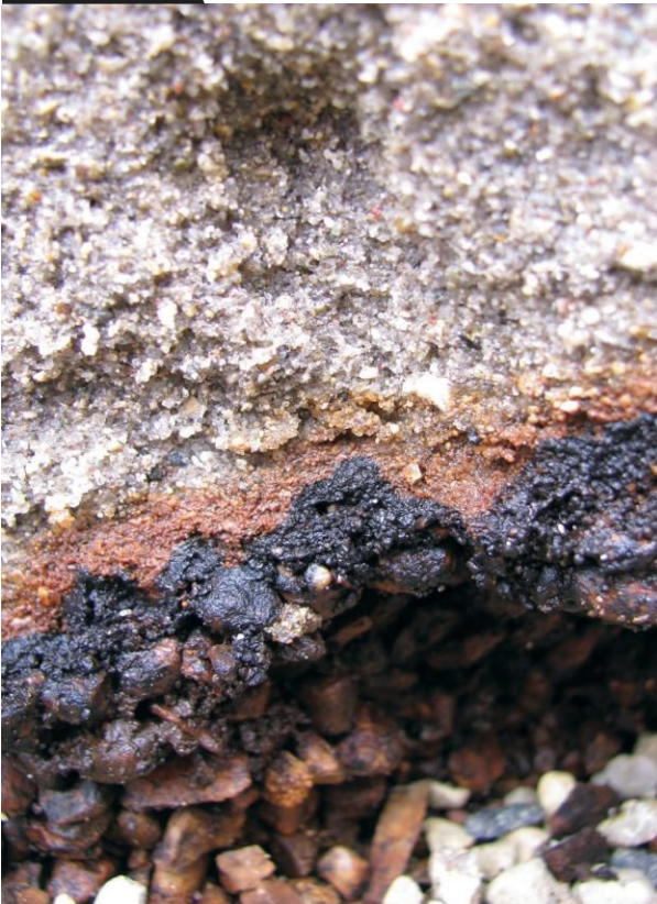
Iron layer in a Wisconsin putting green. The oxygenated pea gravel layer causes reduced iron in the root zone to oxidize at the textural interface. The darker black color is older, strongly oxidized iron; the light orange color is recent, weakly oxidized iron.
