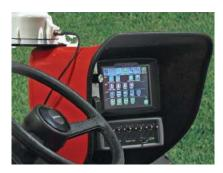
The Capstan® SharpShooter® and the SharpShooter Electronic Control allow a constant operator-set pressure at rates from 0.4 to 5.0 GPT at speeds from 2 to 10 mph.
