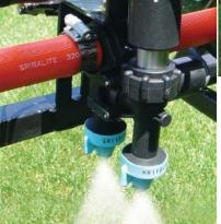
The Star Command System controls the on and off spraying function right at the tip. Shutoff is instantaneous.
