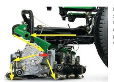
Exclusive rear-attaching point yoke system (red arrow) and adjustable hydraulic down pressure help apply additional force to the rear roller, preventing unsightly rippled lines in the turf.
