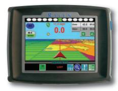
You'll see on the monitor an "As-Applied" map of the application as it is being created by the GPS-guided sprayer's individual nozzles. They will automatically and instantly shut off over areas that have already been sprayed and automatically and instantly turn back on over unsprayed areas. "As-Applied" maps can be created and named for each fairway.
