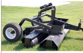
vehicles and windows. Any projectiles picked up by the mower are directed down and backwards, creating a safer environment."
