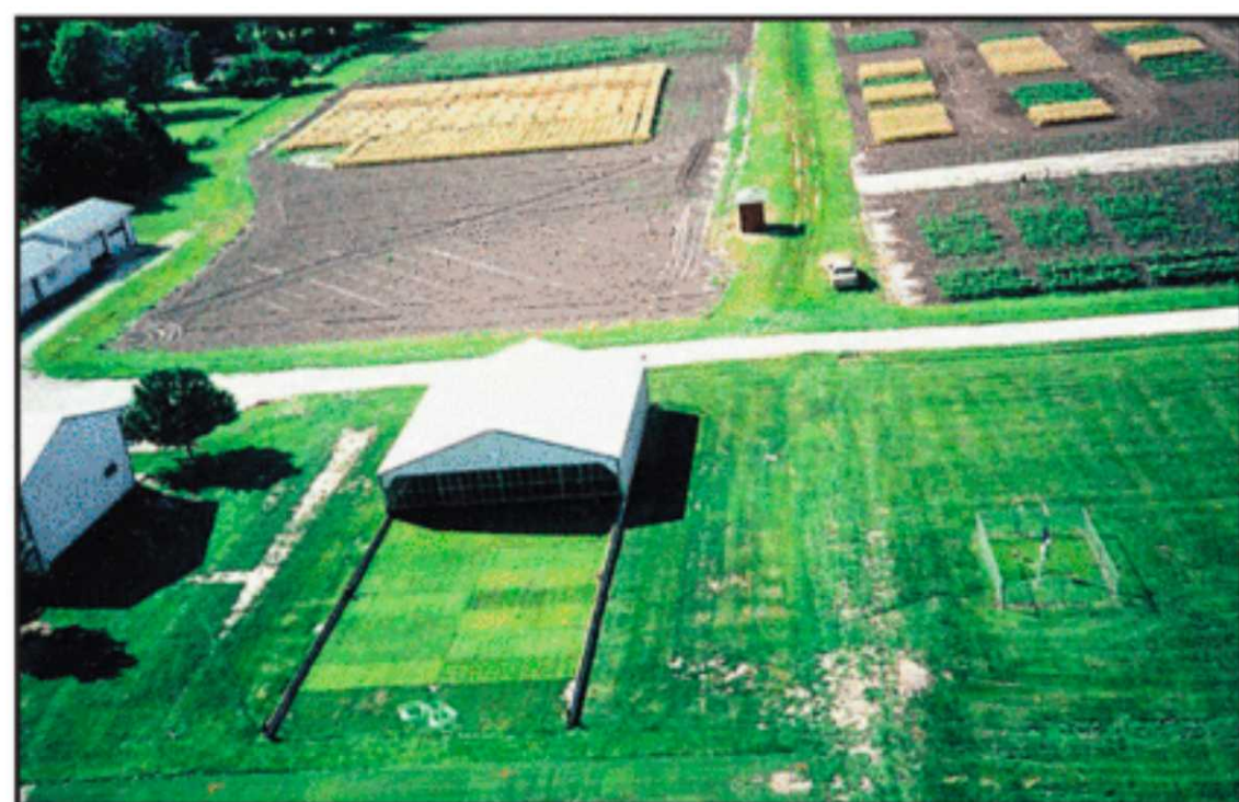
The study explored the impact of deficit irrigation on tall fescue rooting. Evapotranspiration of well-watered turf was measured using small weighing lysimeters. The shelter in this photo was moved to cover plots with the onset of precipitation.
