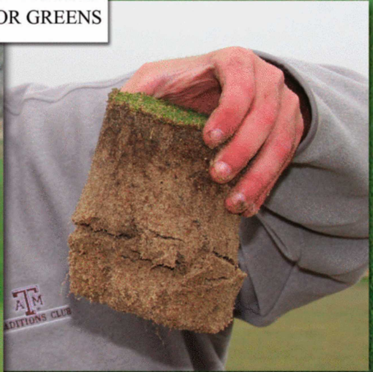
Cup-Cutter Profile from 4-1/2 Year Old Emerald Dwarf Green at Traditions Golf Club
