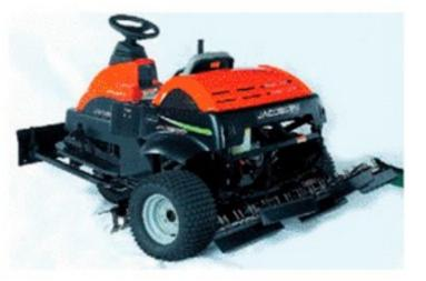
ing steering wheel and a redesigned hydro pedal, it's easy to operate and comfortable to drive. The Groom Master II is available with several attachment options, including a plow, cultivator, rake and scarifier.
