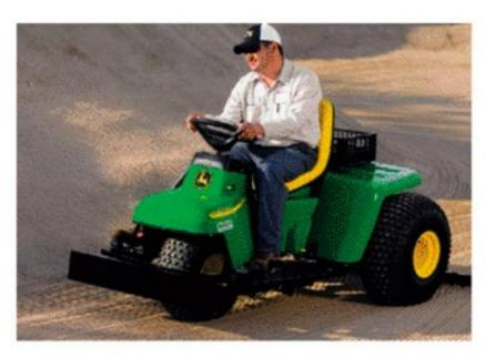
The three-wheeled, self-propelled John Deere 1200A Bunker and Field Rake delivers power, reliability and versatility, according to the company. With features like superior traction, low maintenance and ease of operation, the 1200A provides more machine for the money. Its powerful 9.5-horsepower, aircooled Kawasaki engine delivers efficient
