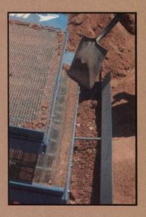
So, what happens to the "undesirable" material being separated from your sand? All material larger than USGA spec, along with clay content, rolls off the back of the screen deck and into the removable waste bin. This allows you to dump your debris in the bed of your utility vehicle, or other receptacle, for disposal later. All that's left behind is the bunker spec sand you originally started with.
