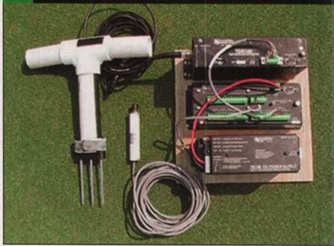
Portable hand-held TDR probe used to measure volumetric water content of the field experiment sites.
