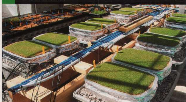
This greenhouse experiment with creeping bentgrass sod grown in calcareous sand on gravel beds simulates a USGA putting green.
