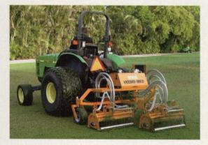
The double-ended blades are tipped for extra durability and the spacing of the blades can be varied by using flexible spacers. The **SISIS VEEMO** has three independently floating heads to closely follow ground contours without scalping, and depth of cut is infinitely variable with a locking micro-adjuster on each unit.
