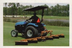
presentation. The brush sections float to follow ground contours. The outer sections fold hydraulically for transport and stands are supplied for storage.
