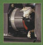
Better than a battery: an alternator powers the reels on the 2500E, giving it consistent power all day long.
