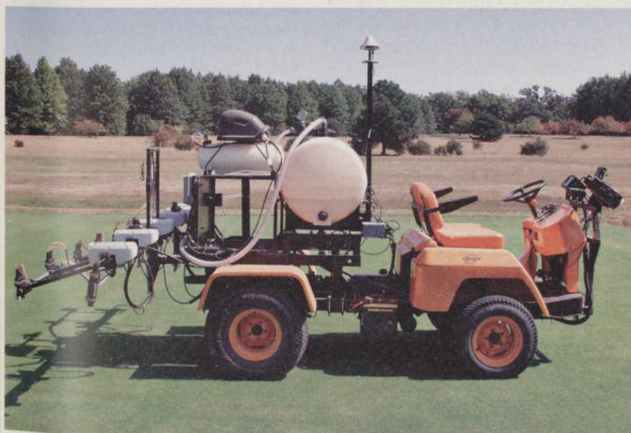
Sensors may be used with a variable rate nitrogen applicator (shown here) to maintain healthy turf by applying prescribed rates in areas as small as 2 square feet.
