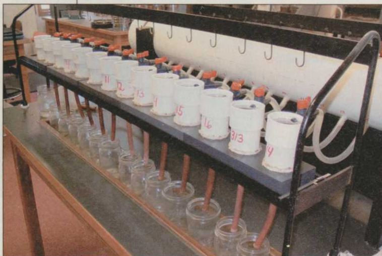
A permeameter test is used to measure the infiltration rates of greens mixes.
