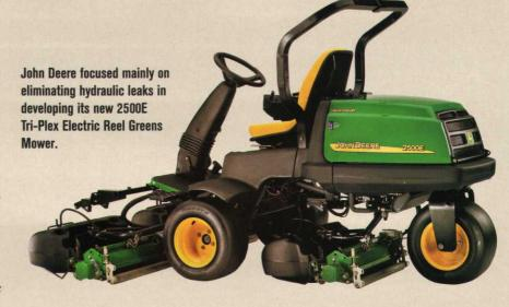
man says, noting that Deere didn't want to sacrifice the power of a gas or diesel engine for an electric engine. "In theory, this machine isn't driven to be quiet. It's about elimination of the hydraulics."
