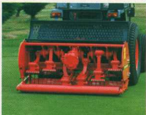
Redexim Charterhouse manufacturers Verti-Drain, the original deep tine aerator.
