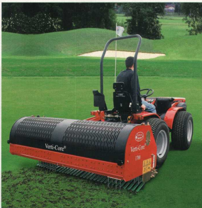
Redexim Charterhouse now offers the Verti-Core, which is available in three sizes and features the proven direct crank drive system for simplicity and durability.
