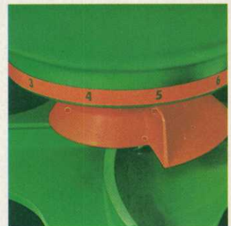
The unique helical cone adjusts to control the spread pattern for particles of different sizes.
