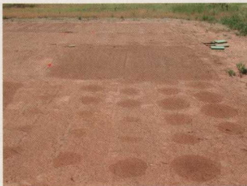
Figure 1. The wetting at each plot was sufficient to see visible wetting patterns on the surface.
