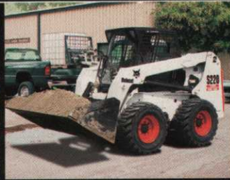
Skid-steer loading topdresser
