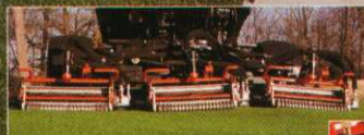
The Super LF-1880's narrow, 18" reels and patented lift arms precisely follow uneven contours.
