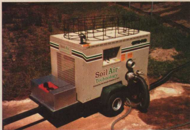
The GTS-RG portable unit is easily transferred between holes.
