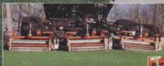
The Super LF-1880's narrow, 18" reels and patented lift arms precisely follow uneven contours.
